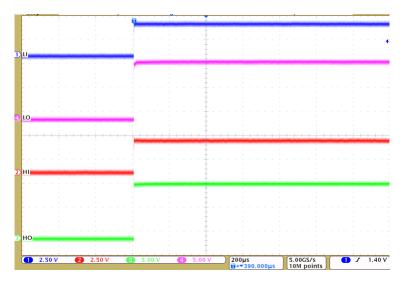
Figure 48. Simultaneously Supported HO and LO High State
