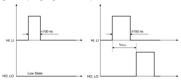
Figure 46. Minimum Turn-On Pulse
