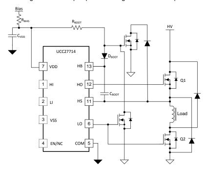
Figure 49. Two-Transistor Forward Converter Circuit
