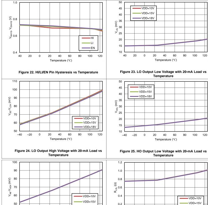
Figure 26. HO Output High Voltage with 20-mA Load vs **Temperature**
