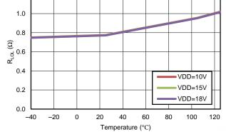
Figure 27. LO Output Pull-Down Resistance vs Temperature
