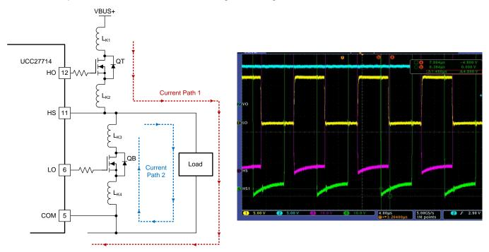
Figure 50. HS Negative Voltage In Half-Bridge Configuration
