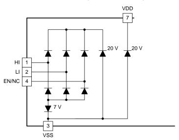
Figure 40. Diode Structure of Input Stage
