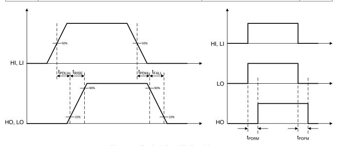
Figure 1. Typical Test Timing Diagram
