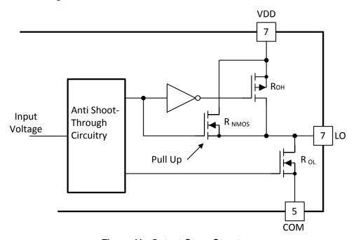
Figure 41. Output Stage Structure
