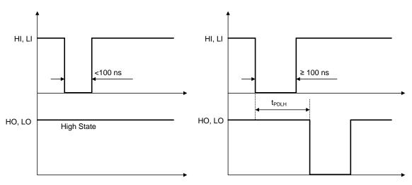
Figure 47. Minimum Turn-Off Pulse
