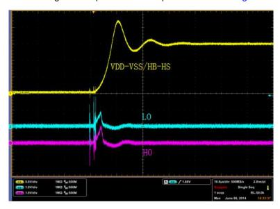
Figure 55. VDD/HB-HS Fast Ramp Up
